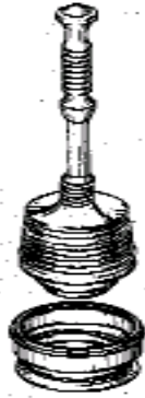
Caption: Example of a design for a plunger type cleaner.
