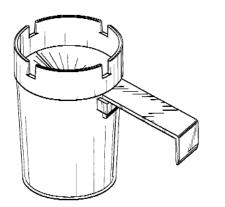
Example of a design for an ash receiver that includes a provision for wall, post or clamp mount.
