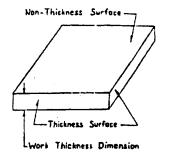
"Nonthickness Surface"; "Thickness Surface"; "Work Thickness Dimension"
