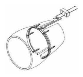
with blocking systems or locking devices, arrangement of locking devices for thrust reversers
