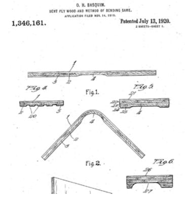
Glued laminated wood which is bent
