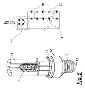
The two dissimilar light sources must be in the same casing or form a single unit
