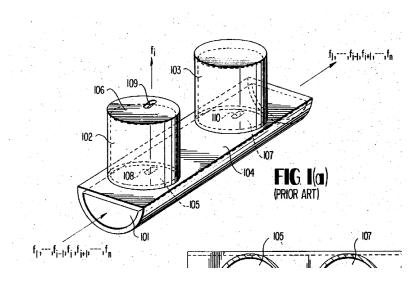
the ferromagnetic material acting as a frequency selective coupling element, e.g. YIG-filters
