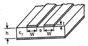
Figure 3.20 Edge-coupled microstrip lines.
