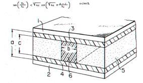
In this figure, 1 and 2 are metal layers, 3 and 4, dielectric layers and 6 is a low loss high dielectric constant dielectric.
