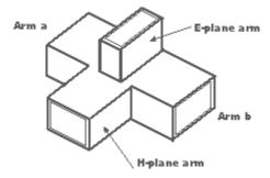
Magic T waveguide junction
