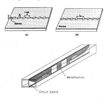
Figure 1. The new E-plane filter.
