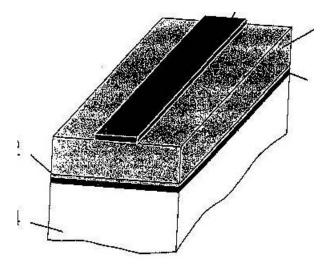
Stripline: A thin conducting strip of width W is centered between two wide conducting ground planes of separation b, and the entire region between the ground planes is filled with a dielectric.
