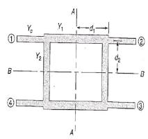
FIGURE 6.29 A branch-line directional coupler.
