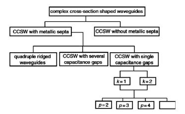
Fig. 1 Classification scheme of waveguides with complex cross-sections
