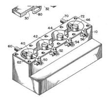
{Comb filters or interdigital filters with metallised resonator holes in a dielectric block}
