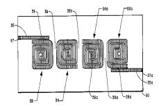
The microstrip ring resonator may be any strip of circular, elliptic or quadrate shape.
