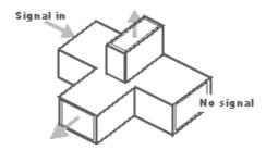
Magic T waveguide junction signal directions
