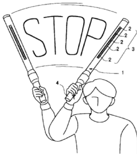
Figure 6 illustrates a baton using light emitting cell array to form a display.
