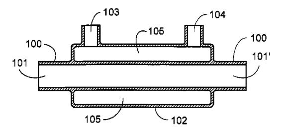
Tube-in-tube heat exchangers with the surrounding tube being closed at one end, e.g. return type, are classified in  $\frac{\text{F28D 7/12}}{\text{F28D 7/12}}$
