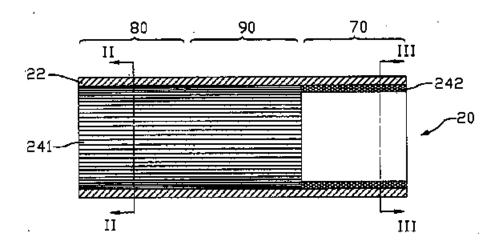
Heat pipes control means (e.g. variable conductance heat pipe).
