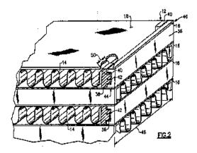
Heat exchangers having conduits formed by spirally-wound plates are classified in F28D 9/04
