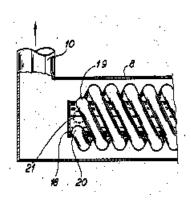
Heat exchangers with spirally coiled conduits are classified in <u>F28D 7/04</u>:
