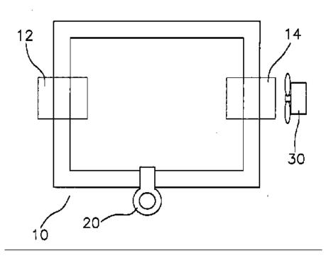
Heat pipes (the intermediate medium evaporates and condenses inside the sealed enclosure) The heat pipes can have a particular shape, e.g. flat tubes. the heat pipes can be formed as a loop, e.g. with separate evaporating and condensing chambers connected by conduits.
