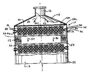
Heat exchangers with conduits being arranged one within the other (tube-in-tube heat exchangers), e.g. concentrically are classified in <u>F28D 7/10</u>:
