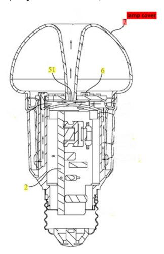
Thermally conductive films or blades contacting the inner surface of the globe to transfer the heat generated by light source to the globe. See illustrative example below:
