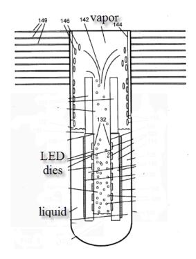
Evaporation and condensation in a housing compartment for cooling of the central arranged electronic circuit:
