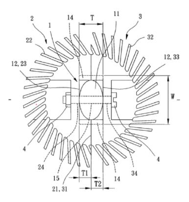
Parallel fins attached to a curved surface, therefore forming an angle with respect to the curved surface:
