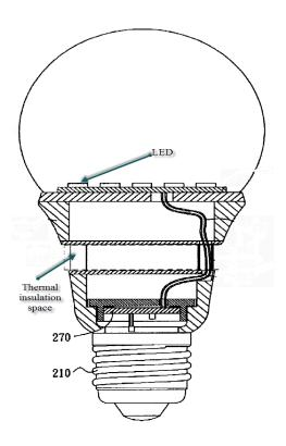
Ilustrative example of air gap between components or in the mass of a component in the figure below:
