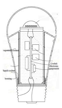
Heat transfer from circuit to the housing, see figure below:
