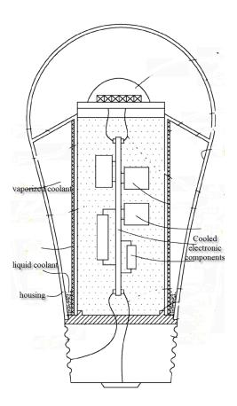
Evaporation of water in open environment to improve heat dissipation:
