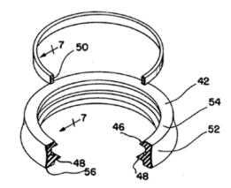
In figures 1a and 1b, note radially directed ribs (46 and 48) of sealing ring (42).
