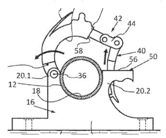
{with two members, the two members being hooked in on one side and fastened together on the other side}
