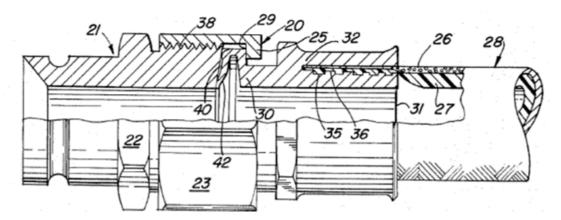
Sealing member (42) adapted to seal by fluid pressure is integral with joint (30).
