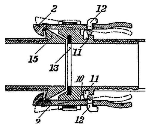
by means of latching members pushed radially by spring-like elements {(radially moved latching members forming a ring F16L 37/0841)}
