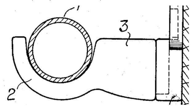
{the member having the form of a closed ring, e.g. used for the function of two adjacent pipe sections}
