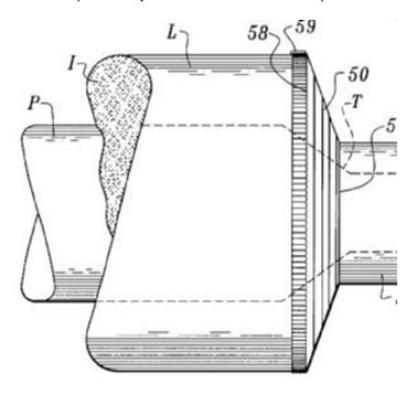
{Joints in which sealing surfaces are pressed together by means of a member, e.g. a swivel nut, screwed on or into one of the joint parts}
