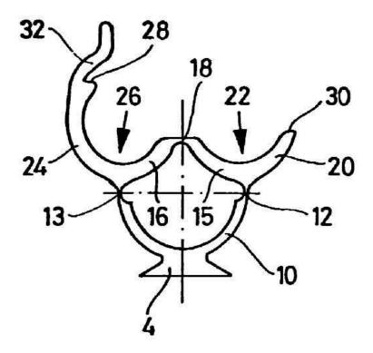
{the ends of the member and the fixing elements being placed on both sides of the pipe}
