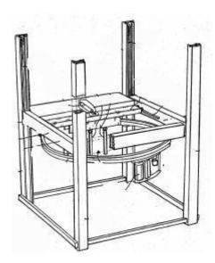
EP1471004 stationary ring type, the dispenser alone moving along the ring
