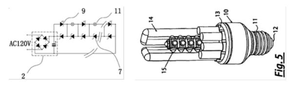
The two dissimilar light sources must be in the same casing or form a single unit.
