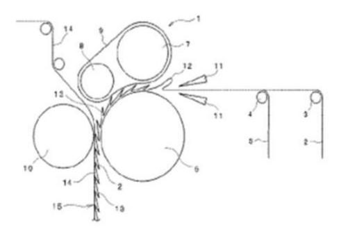
Pleating is a method of an arrangement of fold by doubling the material upon itself and then pressing it into place. The Figure illustrates pleats (13) were formed via rollers (6) and (10).
