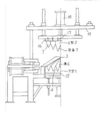
Goffering is the process of creating frills in textile fabrics or wearing apparel so that they are evenly and finely gathered, e.g. make wavy by means of heated goffering iron, or other forms of goffers by pressing or stamping with patterned tools as shown.
