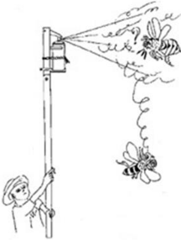
Figure 1 illustrates a pole for use in supporting an aerosol spray container used to exterminate insects, e.g wasps.
