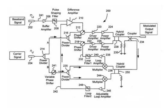
Conversion of angle modulation (212) in amplitude modulation (228).
