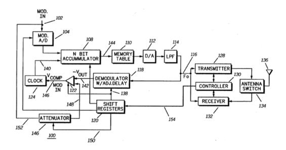
Regulation of mean frequency in a modulator without PLL, using a demodulator in the feedback path
