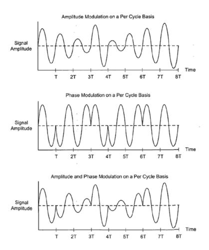
Polar modulation resulting in simultaneous amplitude and phase modulation.
