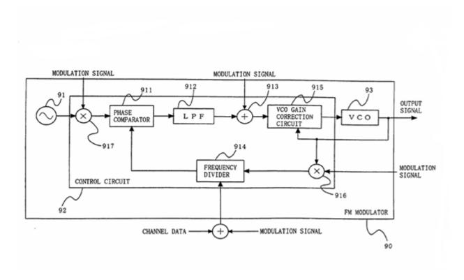
Regulation of mean frequency in a modulator with PLL, using three point modulation (H03C 3/0941) in divider (H03C 3/0925), reference clock (H03C 3/0966) and in front of the VCO (H03C 3/095) and at a mixer (H03C 3/0983).
