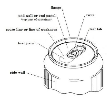
Typical beverage can with a list of its components and terms usually found in the B65D17/00 patent literature.
