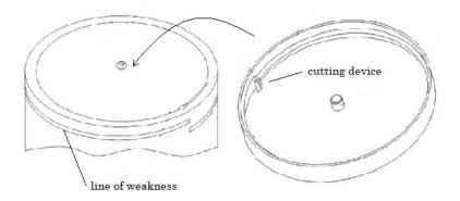
The cutting device is specially adapted to the line of weakness of the container.
