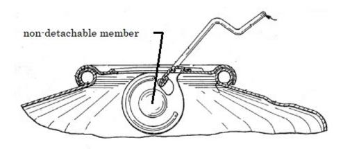
The torn end wall part remains attached to the container.
