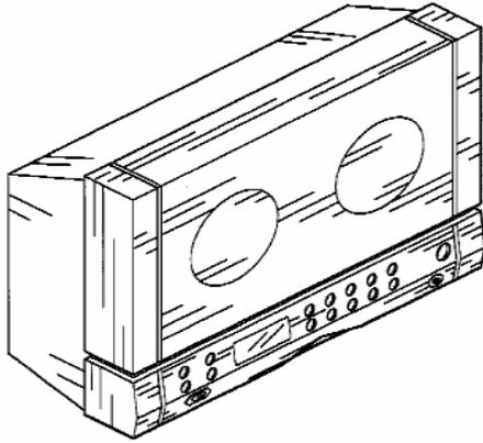
Example of a design for a disc player or recorder with the disc placed vertically.
