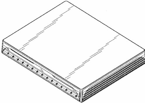
Example of a design for a shelf type cd or dvd player with an array of three or more identical and circular control members.
