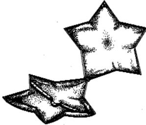
Example of a design for a simulative ash receiver that includes a provision for wall, post or clamp mount.
