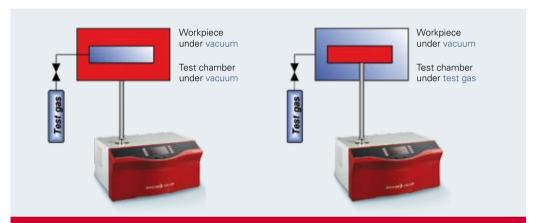
Figure 5.4: Integral leak detection by means of the sniffer and vacuum methods
