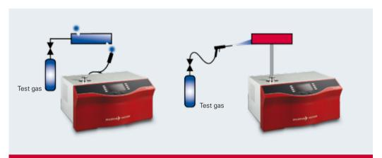
Figure 5.3: Local leak detection by means of the sniffer and vacuum methods
