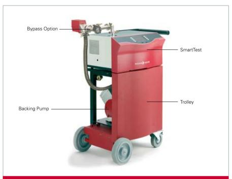
Figure 5.6: SmartTest leak detector, HLT 572 with bypass and dry backing pump XtraDry™
