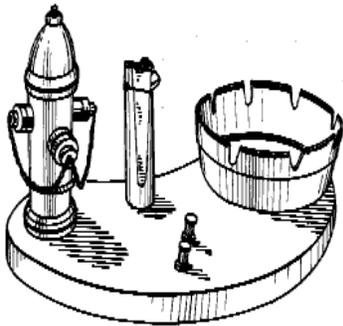
Example of a design for a simulative ash receiver that includes a provision for wall, post or clamp mount and a lighter.
