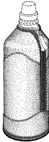
Example of a design for a sheath type holder for a beverage container that includes a closure.
