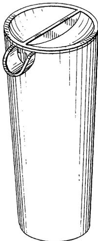
Example of a design with rim-mounted pouring lip with closure.
