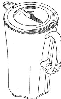
Example of a design for a liquid dispenser with rim-mounted pouring lip and handle attaching plural attachment points.
