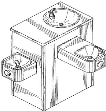
Example of a design with an upwardly directed beverage stream with catch basin.
