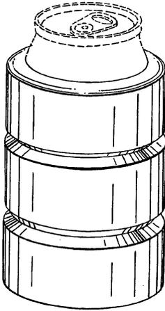
Example of a design for a sheath type holder for a beverage container.
