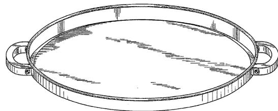
Example of a design for a food server with handles showing plural attachment points.
