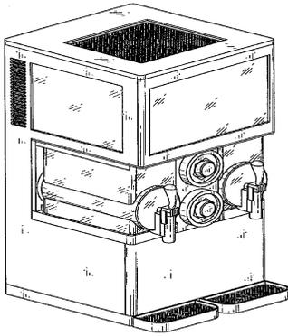
Example of a console type beverage dispenser with plural valve.
