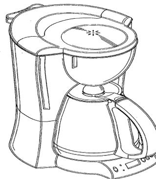
Example of a drip type beverage dispenser with a decanter-warming surface.
