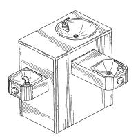
Example of a design with an upwardly directed beveragestream with catch basin.
