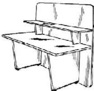
Figure 2. Example of a design for a workstation having uniform thickness and shelf above work surface.
