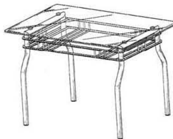
Figure 1. Example of a design for a transparent top table with tubular supports.
