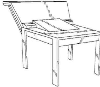
Figure 1. Example of a design for a workstation with shelves above work surface.
