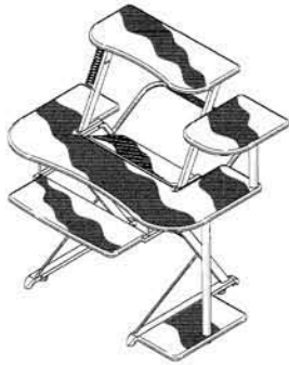
Figure 1. Example of a design for a workstation having shelving above and below work surface with tubular supports.
