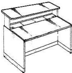
Figure 1. Example of a design for a workstation having uniform thickness and shelf above work surface.
