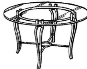
Figure 2. Example of a design for a transparent top table with supports beyond the edge.
