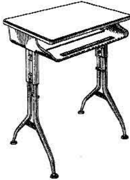
Figure 1. Example of a design for a workstation with tubular supports and shelf below work surface.
