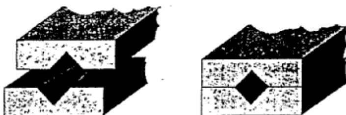
Fig. 1. A diagonal horn made in the split-block technique.
