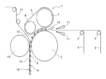
Pleating is a method of an arrangement of fold by doubling the material upon itself and then pressing it into place. The Figure illustrates pleats (13) were formed via rollers (6) and (10).
