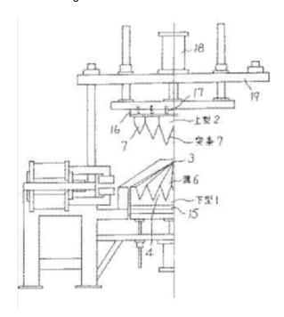
Goffering is the process of creating frills in textile fabrics or wearing apparel so that they are evenly and finely gathered, e.g. make wavy by means of heated goffering iron, or other forms of goffers by pressing or stamping with patterned tools as shown.
