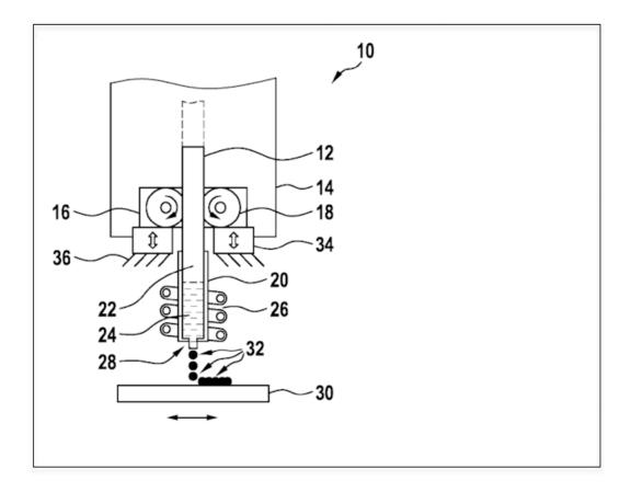
Additive manufacturing using a print head (10) for ejecting droplets (32) of liquid metal (24). The wire (12) in a solid phase (22), is pushed into a melting chamber (20) and melted into its liquid phase (24). At the far end of the melting chamber is an exit orifice (28) for the ejection of gobs (32) of molten wire.
