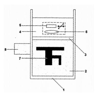
Focused ultrasound additive manufacturing powder bed (2) with ultrasound source (5) and ultrasound optics (6).
