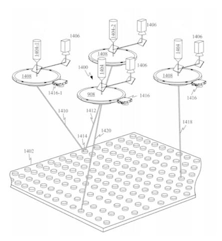
Selective laser melting [SLM] with multiple lasers (1404, 1404-1, 1404-2). Each laser is configured to fuse particles in a defined region of the build plane (1402).
