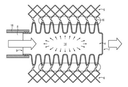
The bellows (4) comprises a pipe connector (8), forming one open end portion (9). The geometry of the bellows (4) makes it flexible and gives it the capability of elongating when a pressure (14) is applied on its internal surface.
