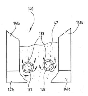
Control of fluidization of powder material (47) comprised in an application device (140) through a fluidization device (131 and 132) integrated within said application device (140).
