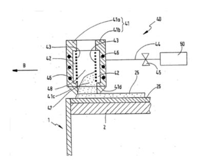
Control of fluidization of powder material (47) comprised in an application device (40) through a fluidization device integrated into the longitudinal walls (41a and 41b) of the application device (40).
