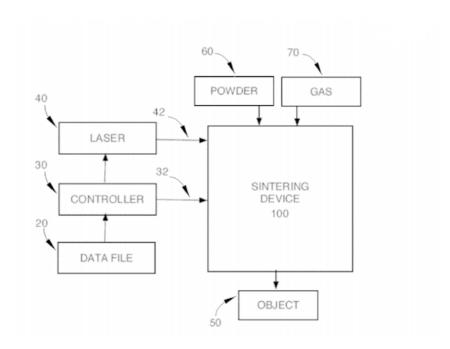
Selective laser melting/sintering [SLM/SLS] by pulsed laser (40) to reduce porosity or microcracks in Al alloys.
