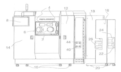
AM apparatus with an interchangeable module (16) incorporating a powder supply and recovery apparatus.
