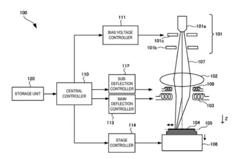
Electron beam melting apparatus (100) with a main deflector (103) and a sub-deflector (108).
