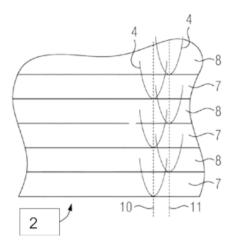
SLS, where a contour position (10,11) of the object (2) is different for different layers (7,8).
