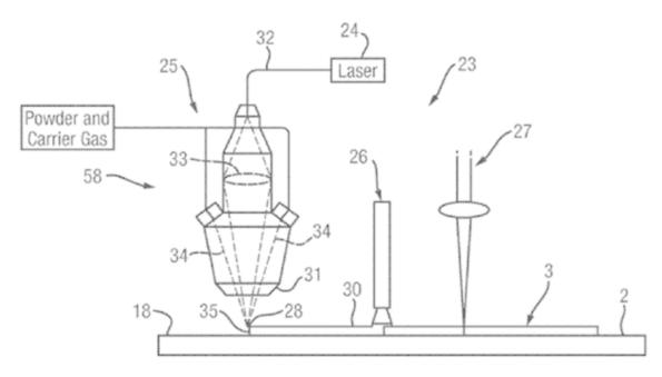
Direct energy deposition (25) of metallic powder with subsequent cryogenic quenching treatment (26).
