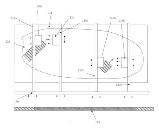
Powder-bed-based additive manufacturing device comprising a movable pair of nozzles (112a and 112b) for blowing an inert gas, and a movable suction device (110a and 110b) for exhausting contaminated gas.
