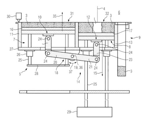
Lever device (14) providing vertical motion of build plate carrier (12) and dose plate carrier (10) in a selective laser sintering melting [SLS/SLM] apparatus.
