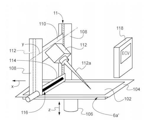
SLM with a laser diode source (112) moving in translation along direction x and vertically by means of cross member (110).
