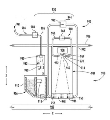
Gantry (916) movable above the build platform (902) having a condensate evacuation subsystem (940) circulating a first gas (946) through the build area (918) and a closed loop subsystem (960) for circulating a second gas (962) over a sensitive component (964).
