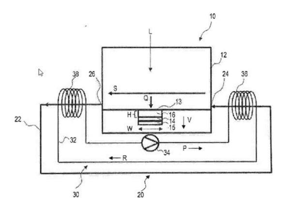
Heating means (36) to heat the process gas.
