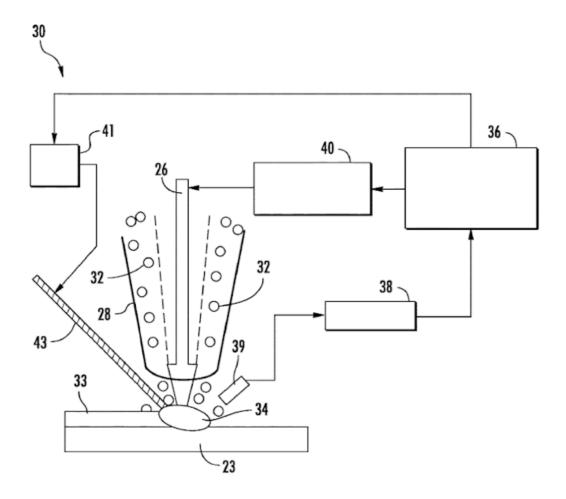
Laser (26), DMD head (28), powder (32) and melt pool (34) are disclosed.
