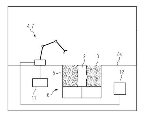
Unpacking device (4) for unpacking article (2) from unsolidified construction material (3).
