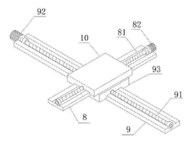
A platform (10) movable in the deposition plane using screw motors (82, 92).
