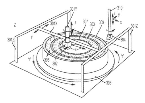
Rotatable build platform (306) for powder bed fusion.
