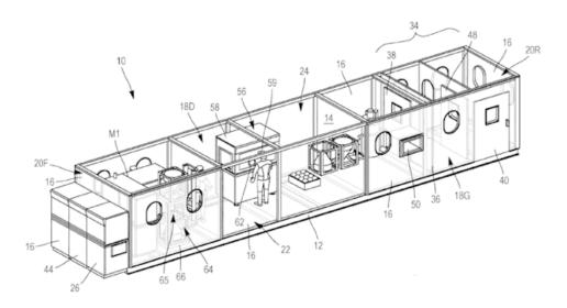
Mobile AM installation (10) with an AM machine (M1) and auxiliary functions.
