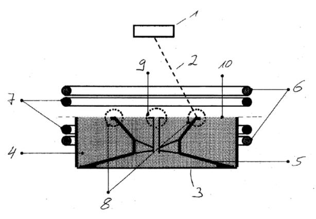
Induction heating coils (6, 7) and heating component (5) in powder bed in container (3).
