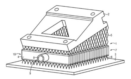
The support structure (1) connects the printed part (2) to the building plate (3). It comprises a first part (6), being arranged on the building plate (3), and a second part (5), being arranged below the printed part (2). The support structure (1) comprises a third part (4) which is arranged at a centre part (10) of the structure part (1), above the first part (6) and below the second part (5).
