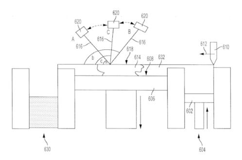
Additively manufacturing a turbine engine component, where grain orientation is controlled by varying the laser (616) irradiation angle (a, b, c) of the galvanometric scanner (620).
