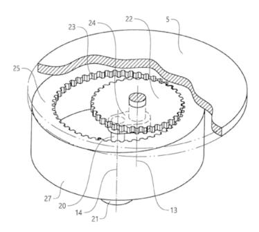
Driving means (20-25) to provide rotation and increase tangential speed at the centre region of the build platform (5) in a selective laser sintering/melting [SLS/SLM] apparatus.
