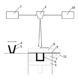
Applying laser shock peening between forming subsequent layers in SLM.
