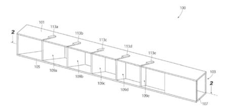
Controlling gas flow above the build plate, where flow filed sensor data is used to modify the flow with the help of actuators (113 a-e) connected to baffles (109 a-e) of an exhaust manifold (100).
