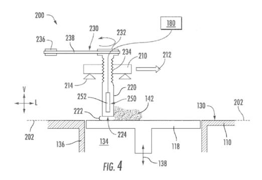
Recoating assembly (200) with a recoater blade (220) movably coupled to a support beam (210).
