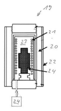
Step 2: Hot isostatic pressing after SLS/SLM to increase the density of the workpiece.
