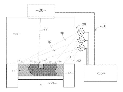
A plurality of image sensors (30, 32, 34) and a processor (56) for combining the fields of view of the sensors to a single image.
