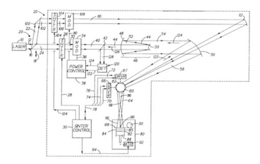
SLM apparatus with a laser source (10) and optics for creating a focused beam (58, 96) and an unfocused beam.
