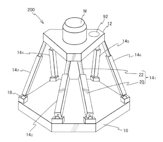
Table (12) for holding workpiece (W), positionable with 6 degrees of freedom by pneumatic control of rods (14).
