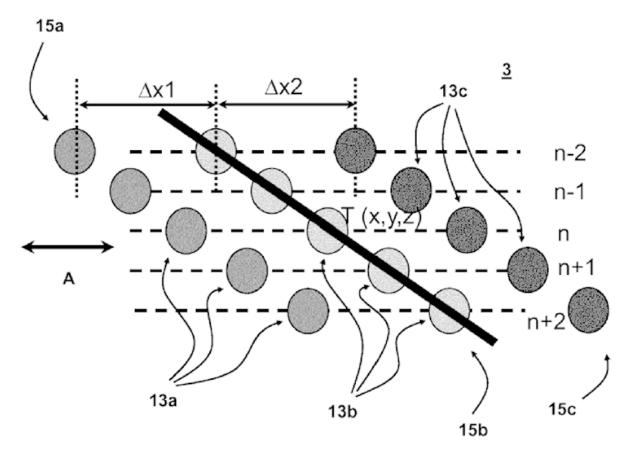
Arrays (15a-c) of beam spots (13a-13c) for both preheating (a) and post-heating (c) in addition to fusing (b).
