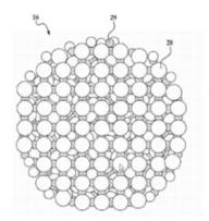
Granules (16) of the build material comprising metal particles (28) bound by a polymeric binder (29).
