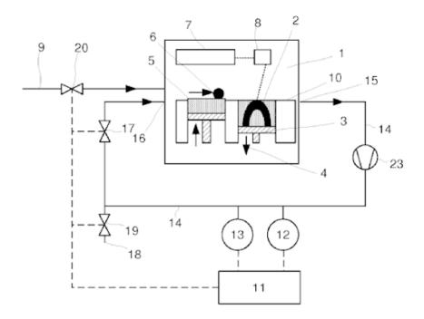
Atmosphere control for SLM using a hydrogen sensor (12) and an oxygen sensor (13) for controlling the atmosphere in the processing chamber (1) based on the sensor values.
