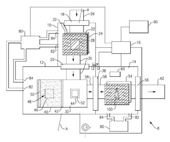
System (8) where a component (100) is formed in the chamber (12) and undergoes post-processing in the chamber (14). It is transferred between the chambers (10, 12, 14) by means of belt or conveyor (30, 58, 62).
