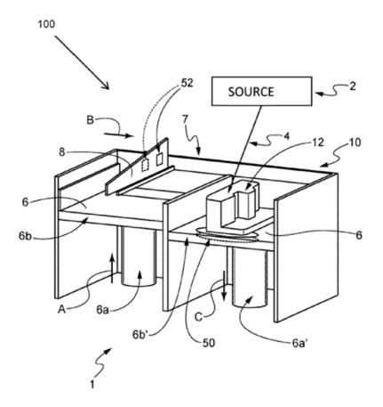
Induction system (50) to heat the build platform (6b').
