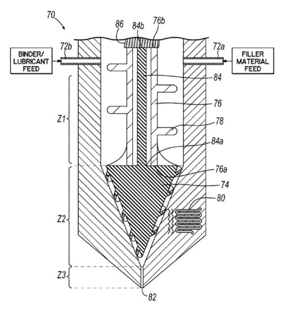
System assembly (70) for extruding material, comprising a binder and a filler. The assembly (70) comprises a mixing device (76, 78), a heating device (80) and an outlet nozzle (82).
