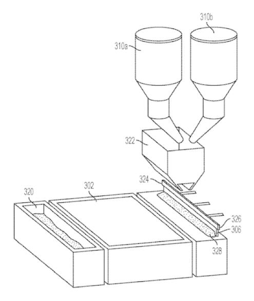
Powder bed device comprising a first powder reservoir (310a) with a first powder composition and a second powder reservoir (310b) with a second powder and a dispenser (322) for receiving a blend of the first and second powder according to a desired composition of the blend.
