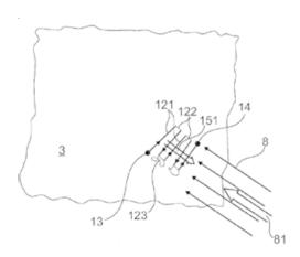
Controlling shielding gas flow direction (81) dependent on, e.g. the direction of scanning (151).
