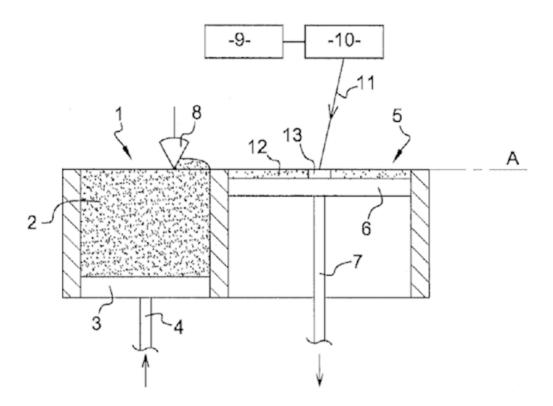
Selective melting in powder bed using laser or electron beam (11).
