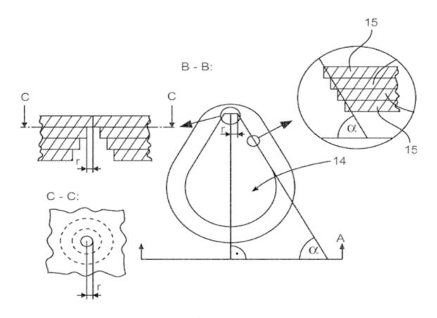
A method for manufacturing a component having an overhang, wherein a local build-up angle ( $\alpha$ ), which occurs between two consecutive layer sections (15) of an overhang, does not fall below a predetermined minimum build-up angle to the base layer.
