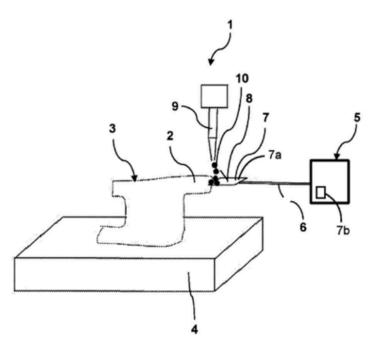
Support device (5) with at least one movable support arm (6) for temporary holding of at least one support element (7) arranged on the support arm during the additive manufacturing of a particular component (3) above the building platform (4).
