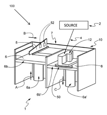
Illuminators (52) to preheat the powder in the powder bed (6), where the manufacture of the workpiece (12) takes place.
