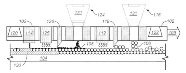
Printhead (102) for powder bed devices comprising means for feeding material (131).
