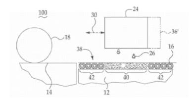
Binder jetting comprising selectively depositing a patterning fluid (26) onto granules (16) of build material.
