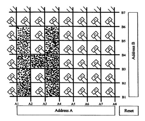
Programmable planar LED light source matrix for curing binder in a metal powder bed to bind the metallic powder in a selected area (H) at once to increase the build speed compared to a point-by-point illumination.
