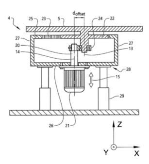
Driving means (20-25) to provide rotation of the build platform (5) in an SLS/SLM apparatus.
