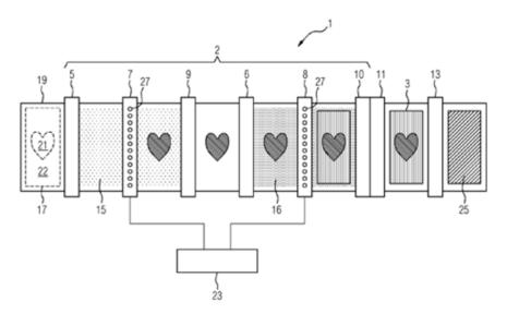
Additive manufacturing apparatus (1) with deposition (5), fusing (7) and powder removal (9) units for first material (15) and corresponding units (6,8,10) for second material (16), followed by sintering (11) and coating (13) units.
