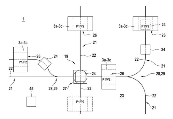
Plant (1) with several machines (26) with process stations for preprocessing (3a), additive manufacturing (3b) and post-processing (3c).
