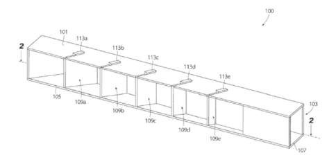
Additive manufacturing system comprising an exhaust manifold (100) with baffles (109a-e) movable with actuators (113a-e).
