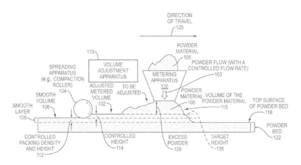
The powder material (105) is metered onto the top surface (118) of the powder bed.
