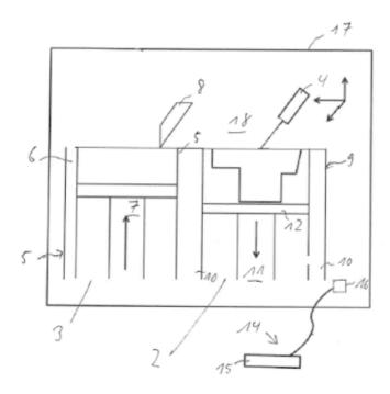
Step 1: Manufacture of a workpiece by selective laser sintering/melting [SLS/SLM].
