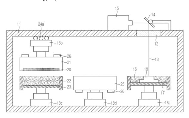
Compacting plate (25) for compacting layer (20) in dosing device (21) before application of layer (20) on powder bed (16).
