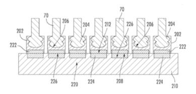
Build platform (210) for powder bed based additive manufacturing gas turbine blades (70) comprising component fixtures (202) for holding worn air foils.
