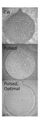
Comparison of pulsed wave/continuous wave laser [CW] for Al alloys reduction of microcracks with pulsed wave laser.
