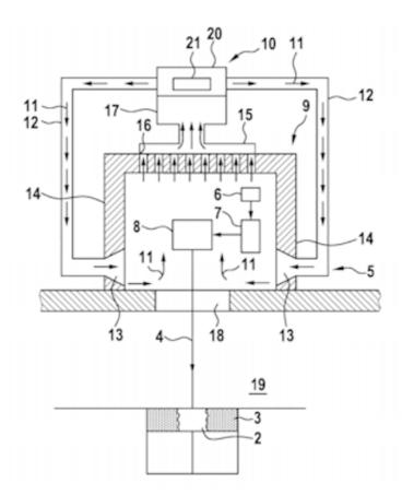
Housing (9) for irradiation device provided with stream inlet (13) and vents (16) for generating a gas stream.
