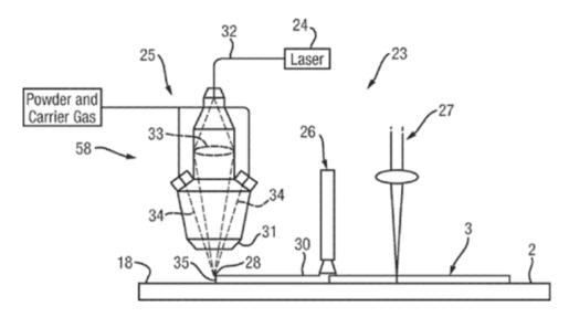
Direct energy deposition (25) of metallic powder + cryogenic quenching treatment (26) + laser shock peening (27).
