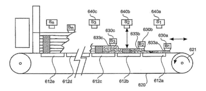
Substrates (612a-e) in translator movement within deposition plane.
