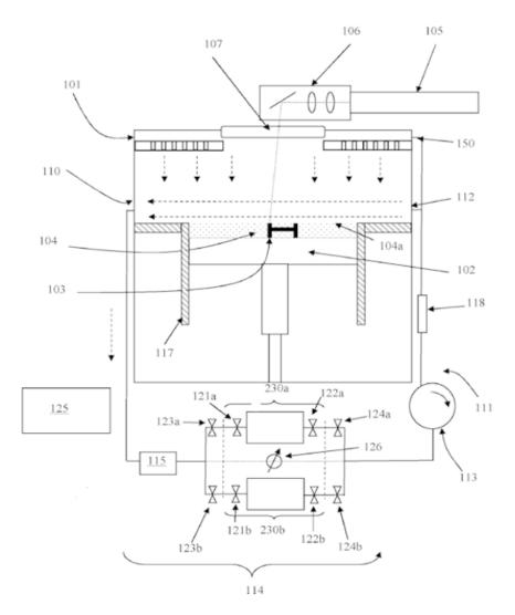
SLS/SLM apparatus with filter system (114). Process emissions, such as spatters and condensates are removed from the process gas by the filter system (114) before gas recirculation within the build chamber (101).
