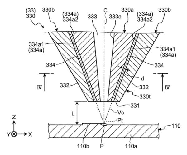
Nozzle for direct metal deposition of metallic powder onto the surface of a base (110a) or onto the surface of an object (110) with constant gap (d) between body component (330a) and (330b) of the nozzle.
