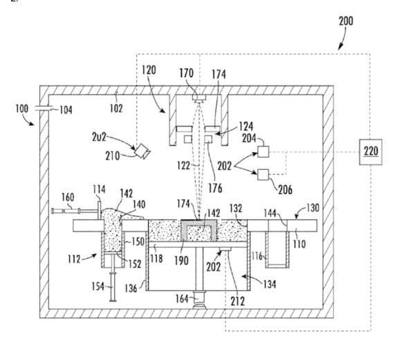
Electron beam (122) melting in powder (142) bed.
