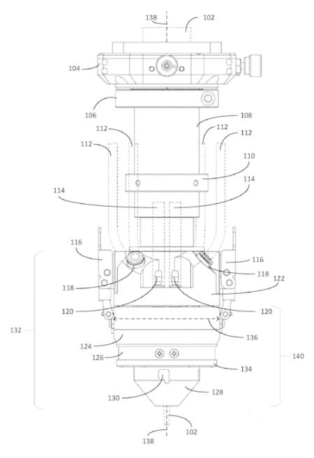
Laser metal deposition head (132) comprising a nozzle assembly (140). The powder is provided to powder inlets (118) and guided through the nozzle assembly (140) to the focal point of the laser beam (102).
