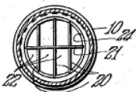
Figures 1a, 1b and 1c illustrate fins (20, 30) acting as flow straightening means to reduce turbulence.
