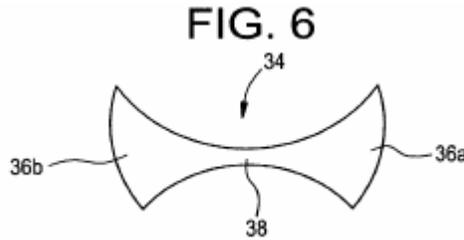
opening **34** comprises large openings **36a** and **36b** and a restricted opening portion **38** between **36a** and **36b**. It was found that the restricted opening portion **38** still allows sufficient outflow of heated air to sufficiently soften the overlapping portion of the thermoplastic sheets over and under the fastening means in order to weld the thermoplastic sheets together over the interposed fastening means.
