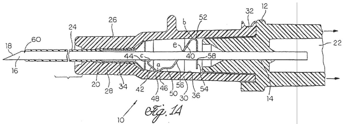
Woehr describes Figure 1A as depicting catheter 10 including needle hub 12, needle 16 with needle tip 18, catheter hub 26, and needle guard 40 in the form of a unitary spring clip. *Id.* at 4:8–28, 50–51. Functionally speaking, as needle 16 is withdrawn from a patient, needle guard 40 “automatically snaps into a retracted position” to block needle tip 18 to prevent accidental contact to the health care practitioner. *Id.* at 4:43–49.
