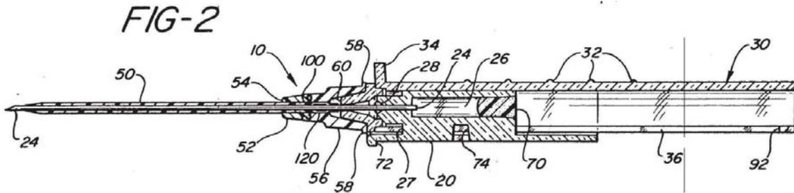
Figure 2 depicts a cross-sectional view of Van Heugten’s catheter assembly 10. *Id.* at 2:9–10, 19–21. In particular, Figure 2 illustrates catheter assembly 10 with catheter 50 and needle 24, which needle guard 30 covers upon retraction of needle 24 to prevent inadvertent needle injury to the user or others. *See id.* at 2:36–39, 3:34–58. Catheter assembly 10 also includes valve membrane 110, which is illustrated in Figures 4a and 4b, which we also reproduce, below:
