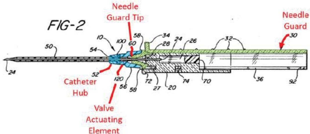
Figure 2 of the catheter hub assembly from Van Heugten, above, and as annotated by Patent owner, illustrates in green a portion of the needle guard and, in blue, the catheter hub.
