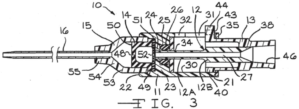
Figure 3 of Rogers illustrates check valve assembly 10 including slit 48 in valve 14, and sliding separator 12, in comparison with Figure 2 from Tauschinski below.
