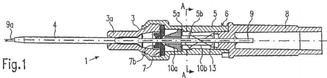
According to the '762 patent, Figure 1 depicts catheter insertion device 1 with catheter 4, needle hub 8, to which hollow needle 9 is fixed and which needle 9 passes through valve disc 7 and extends through catheter 4.
