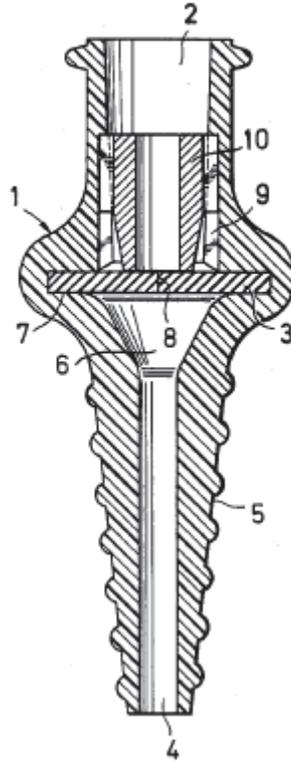
Tauschinski's valve, shown above in Figure 2, includes valve disc 3, slit 8, and slidable actuator 10.
