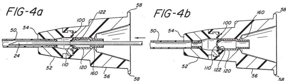
As disclosed in Van Heugten, Figures 4a and 4b further show membrane assembly 100 comprising a one-directional valve membrane 110. *Id.* at 3:59–64. Figure 4a (above-left) depicts membrane 110 as being “punctured” by needle 24 (*id.* at 3:59–4:3), while Figure 4b (above-right) depicts needle 24 removed, where upon “removal from the catheter hub 52, the valve membrane closes” (*id.* at 4:6–9). The sealed valve member 110 is “generally configured as a ‘duck bill’ valve or a valve of similar
