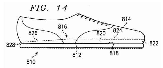
Figure 14 depicts a shoe with an outsole affixed to a shoe upper and an insole which lies over a surface of the outsole enclosed by the shoe upper.
