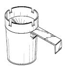
Example of a design for an ash receiver that includes a provision for wall, post or clamp mount.
