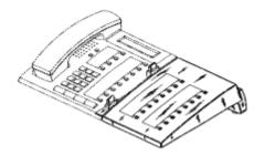
Example of a desktop switchboard with a provision for telephone set.
