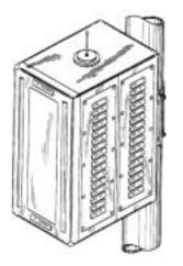
Example of a design for a pole mounted telephone module.
