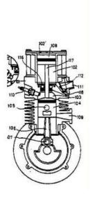
the rear face of working piston acting as pumping member and co-operating with a pumping chamber isolated from crankcase, the connecting-rod passing through the chamber and co-operating with movable isolating member
