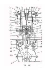
Engine with pulled con-rods during working stroke.
