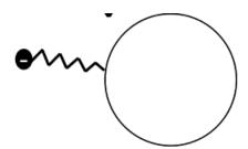
This drawing illustrates e.g. the covalent attachment of a chemical group (might be an alkylene chain) with a terminal negative charge (might be an anionic SO3- group) to the surface of a pigment, e.g. to improve dispersibility. The organic pigment particle is here represented by the ring at the right.
