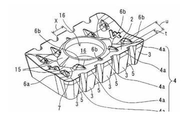
Milling insert with sloped cutting edges (6a-d) and rake faces (10) above a central surface (9):
