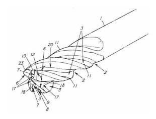
Milling cutter with head detachable from shaft:
