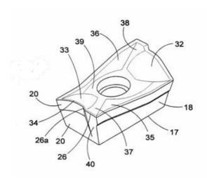
Milling insert with interrupted cutting edge and chip-breaking projections on the top surface:
