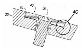
Plate-like cutting insert (10) having a special shape and clamped by clamping member (20) acting almost perpendicular (14) on the cutting face:
