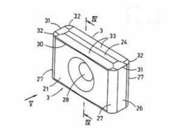
Milling insert with curved cutting edge and wiper:
