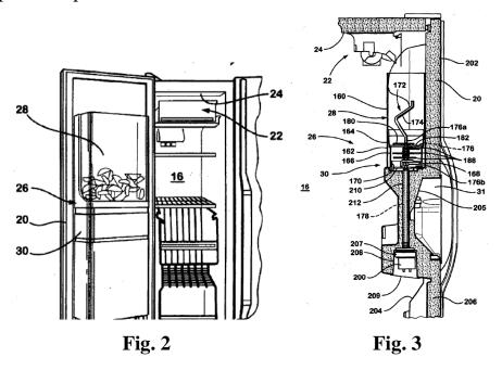
Figure 2, reproduced above left, is a fragmentary perspective view of a refrigerator including the ice maker 22 and the ice storage receptacle or bin 28. Figure 3, reproduced above right, is a fragmentary, side sectional view showing ice maker 22 and bin 28.
